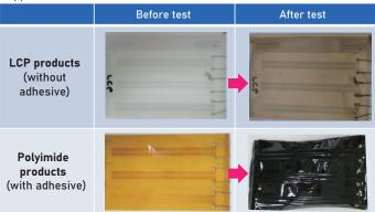
[Measurement of insulation resistance value (n = 3)] (Standard value:  $5.0 \times 108 \ \Omega$  or more)
