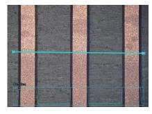
Specifications of products Number of layers: 4 Line & space: 200 µm/200 µm Copper thickness: 85 µm Number of turns: 100
